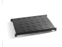
Adjustable shelf for rack cabinets up to 1000mm deep, with 4 post fixing, for supporting equipment that is not designed for 19" rack mounting.
